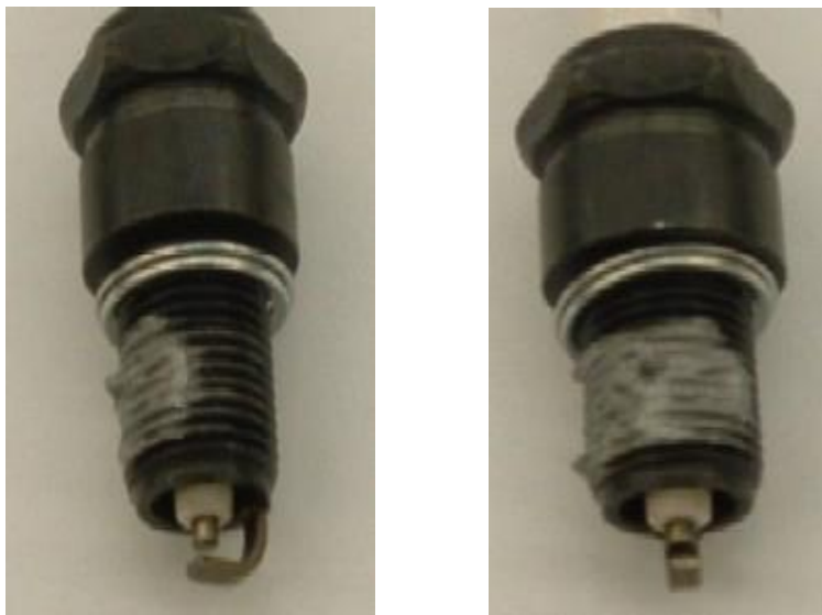
Example of spark plugs that do not have metal shell plating
